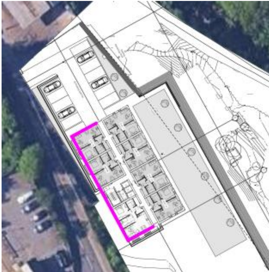
Figure 6.1 – Façades Requiring Additional Sound Insulation Measures
